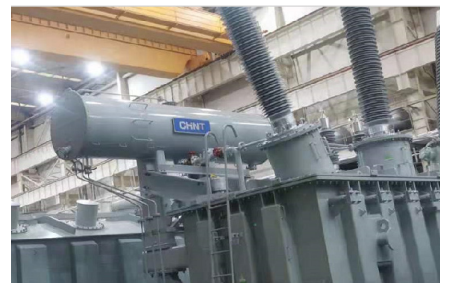
110kV 40MVA Power Transformer to Enersis, Chile
