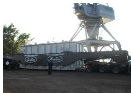
400kV 400MVA Transformer to EMS, Serbia
